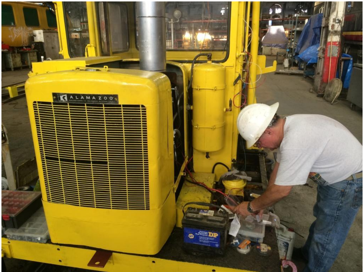
Mike H. continues his tireless efforts at restoring the electrical system of the Kalamazoo tug
